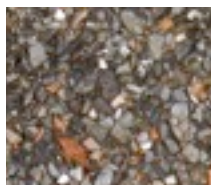
chip seal, small aggregate in binder - consider different colors & rock types - bluestone gravel, pea stone, crushed granite
