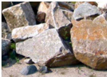
Igneous rock: granite local granite is often available recycled as rectangular cut blocks for seating, old curbstones for edges, or cobbles to make paths
